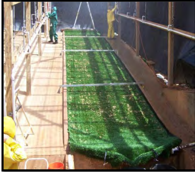
Figure 3 – Rainfall Erosion Control Testing on ClosureTurf® (3H:1V Slope)
