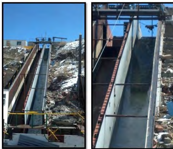
Figure 5 – Steady State Hydraulic Testing of ClosureTurf® with HydroBinder® at CSU
