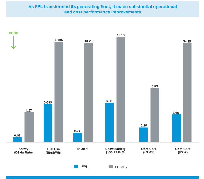
FPL's fleet improvements in safety, fuel efficiency, reliability and cost are integral to more cost effective generating electricity for customers
